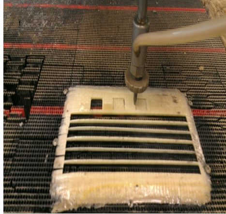
Figure 3.5. Cutting samples for determination of the fiber volume fraction
