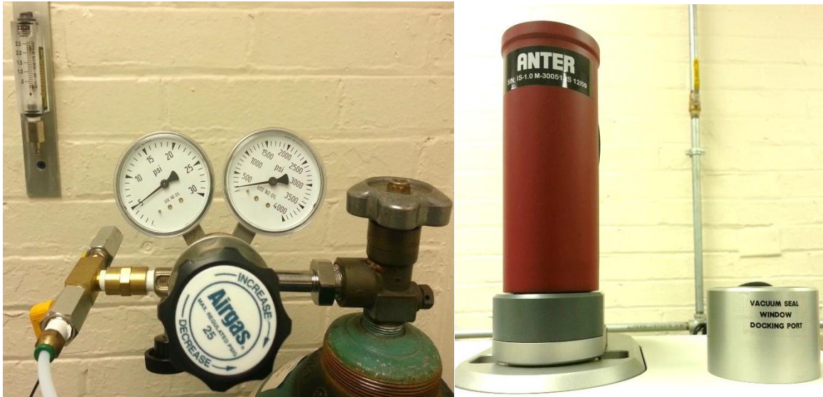
Figure B.14. Compressed Nitrogen Gas and Liquid Nitrogen Indium Detector
