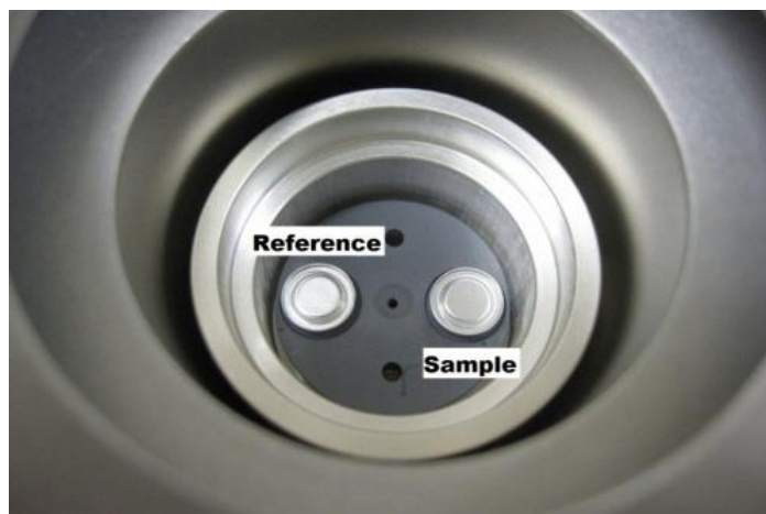
Figure 4.10. Crucibles Placed on the Heat Flux Sensor
