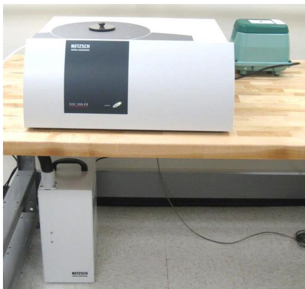
Figure 3.4. Experimental Setup of the DSC 200 F3 Maia® and Intracooler
