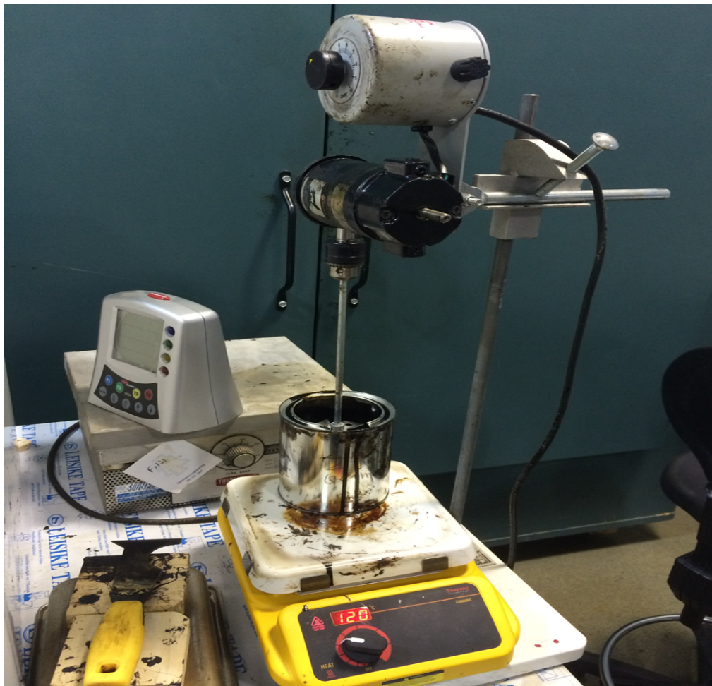
Figure 4-4. The Bench-top High Shear Mixer Used for Blending
