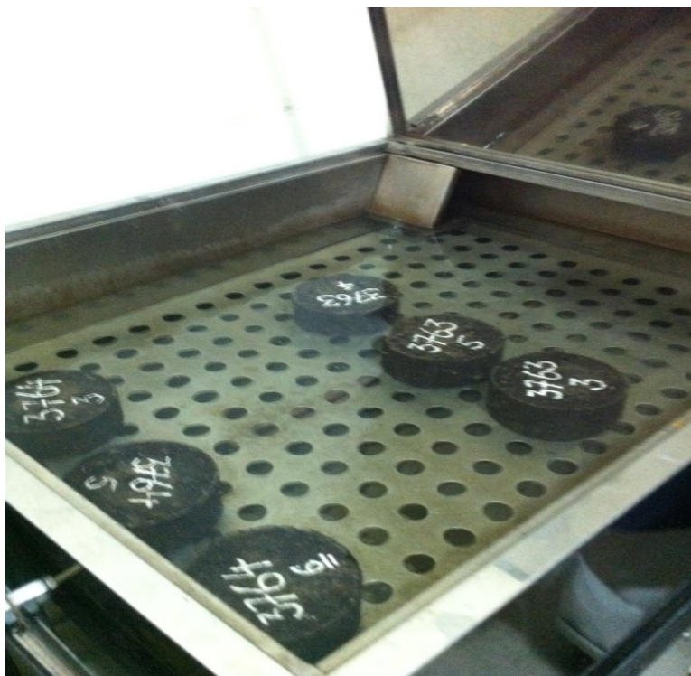
Figure 3-2. Asphalt Mixture Sample Replicates
