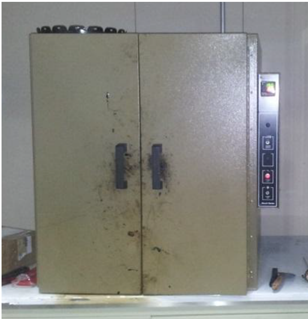
Figure 4-3. Conventional Oven to Heat the Sample
