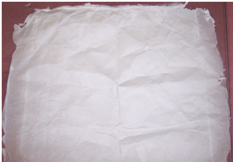
Figure 2.4. Electrospun TEOS nanofibers on a Teflon Sheet
