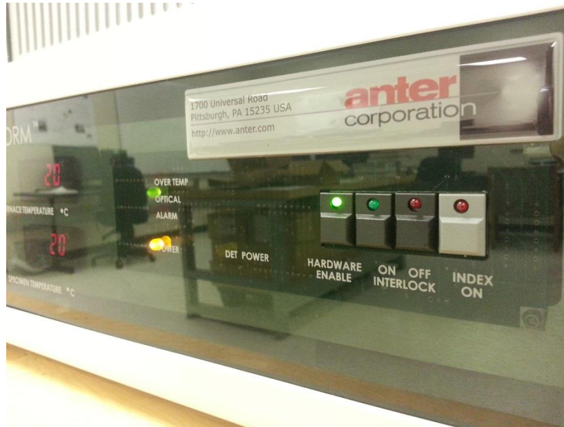
Figure B.6. Hardware Interlock Enable on the FlashLine™ Apparatus
