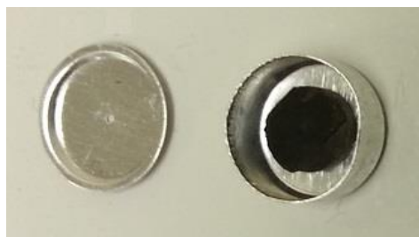
Figure 4.9. Specific Heat Sample Specimen of AS4/3501-6
