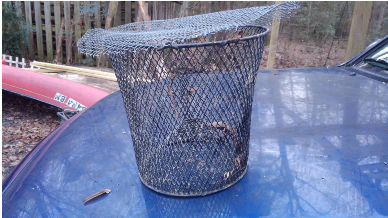
Figure 11. Example of a potential bait retention device to put in catfish pots. The wire top would be cut small so it fits inside the circle on the open end and held in place by a bungee cord.
