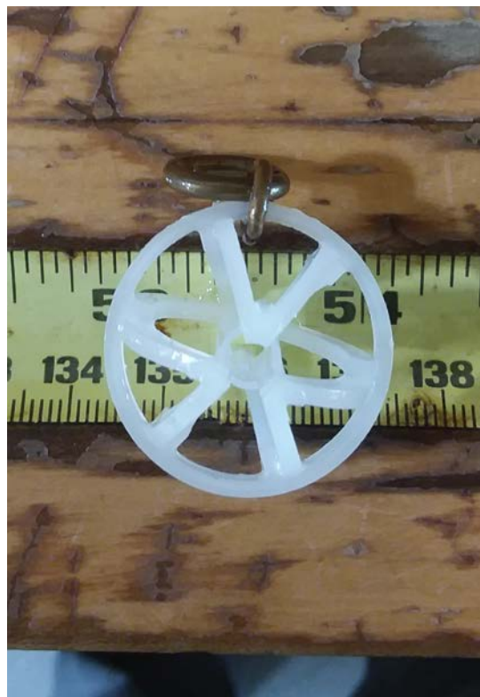
Figure 6. Image of a BioRing used to simulate catch in the scale survey dredge. Each BioRing either had a weight in the center of the ring or a weight attached to the outside of the ring, as shown in this picture.
