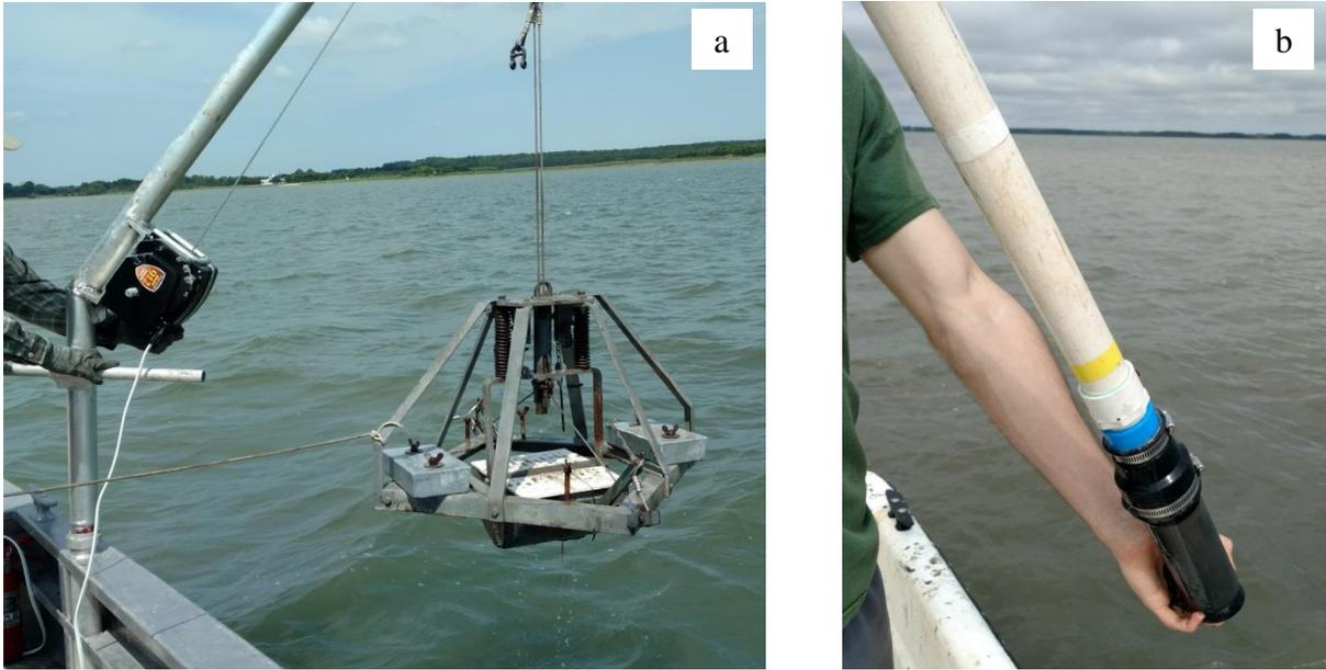
**Fig. 6-3-3** Gear used to collect a) grab and b) push core samples; subsamples from these were collected for surficial sediment organic matter and chlorophyll-a.
