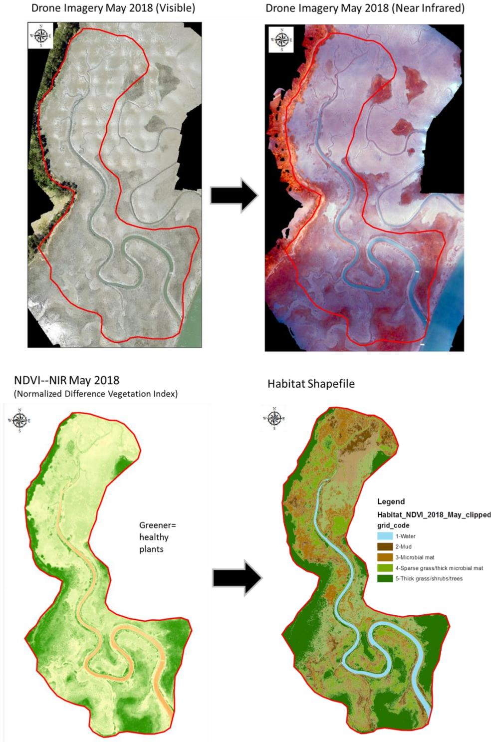
**Fig. 6-2-3.** Visible and near infrared orthomosaics collected in 2018. The specific study area is the red polygon. Imagery was clipped by this study area and post-processed using an NDVI algorithm which ultimately was used to create an ArcGIS shapefile for analysis.
