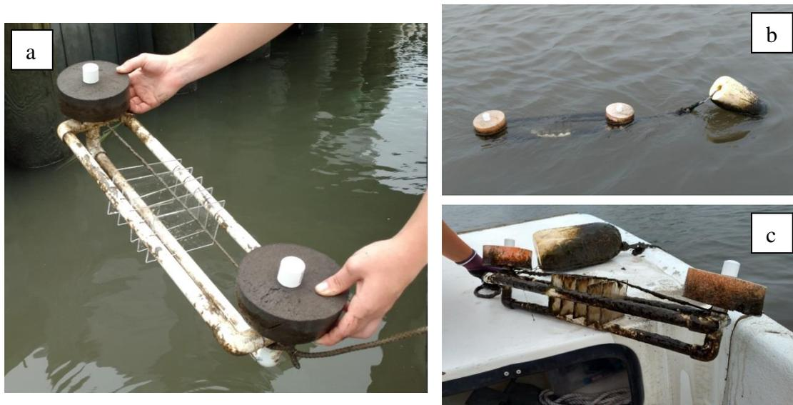
**Fig. 3-2** Biofilm array a) before, b) during and c) after deployment.
