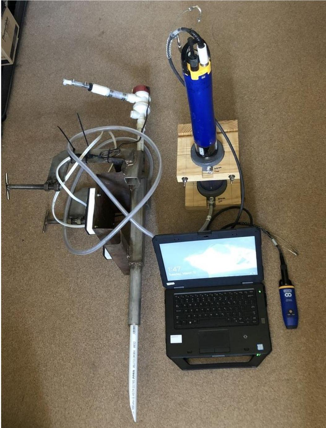
**Fig. 2-2-1** Data flow setup. Transom mount hydraulic ram and bilge pump (left) to send water to a YSI Exo2 Datasonde with a flow cell held in a wooden bracket (upper right), cabled to an ExoGo GPS antenna and data integrator (lower right) to send by blue tooth georeferenced sonde data to a laptop.
