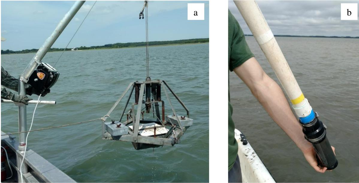
**Fig. 5-1-1** Gear used to collect a) grab and b) push core samples. Subsamples from these were collected for surficial sediment organic matter and chlorophyll-a.
