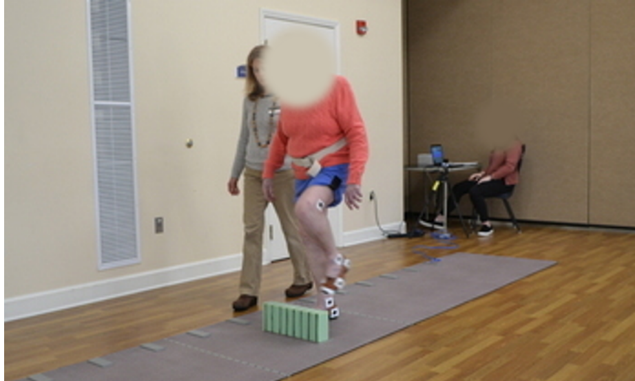
Figure 1.2: The experimental setup for the Williamsburg Landing research. Black dots shown on the subject's legs are used for video gait tracking
