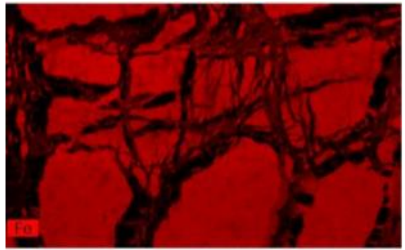
Figure 48: XRF image showing the distribution of Fe in sample 43018.1B
