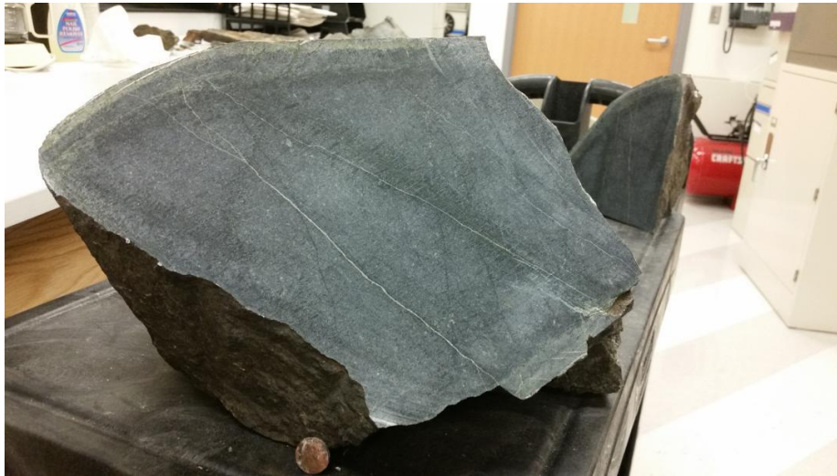
Figure 22: Sample 50218.1B in hand-sample. Penny for scale. Hand-sample is roughly 45 cm to a side.
