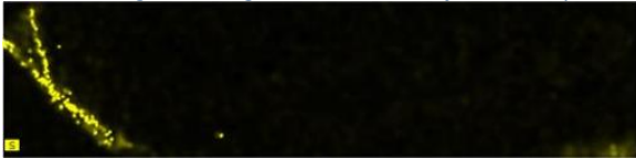
Figure 93: XRF image showing the distribution of S in sample 50218.1B
