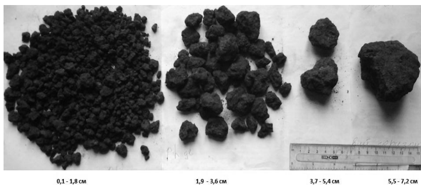
Fig. 4. The fractional composition of the ferrum concretions forms in the ABg horizon of the mollic gley soil
