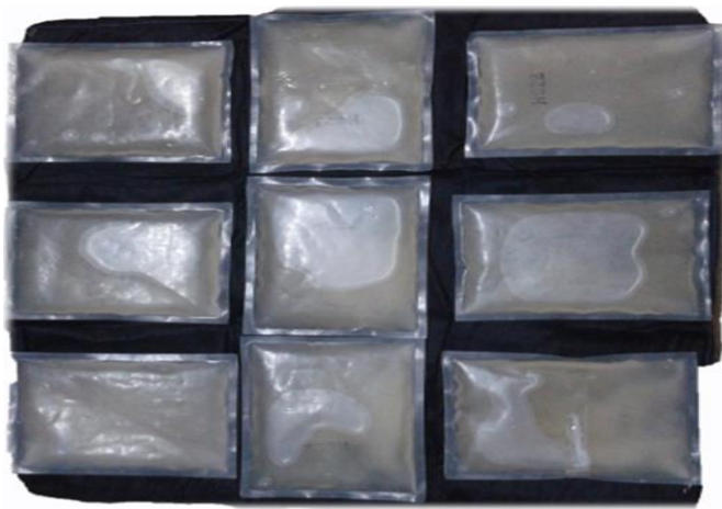
Figure 4. Arrangement of PCM pouches in the cold seat pad
