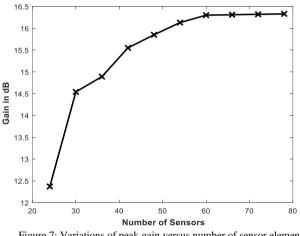
Figure 7: Variations of peak gain versus number of sensor elements
