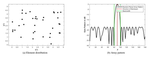
Figure 2: Random planar array pattern and its element distribution
