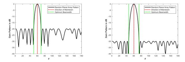
Figure 3: Random planar array patterns with optimum beamwidths for minimum sidelobe level=-20dB (left) and -30dB (right)
