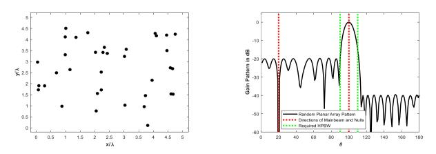
Figure 4: Random planar array pattern with asymmetric sidelobes and a single null control
