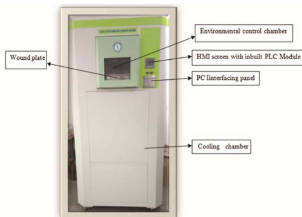
Fig. 2 — SITRA fluid handling capacity tester (SFHCT)
