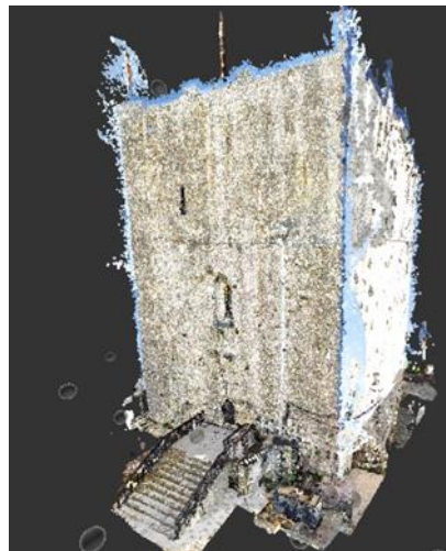
Figure 9. 3D laser scanning of the Tower.
