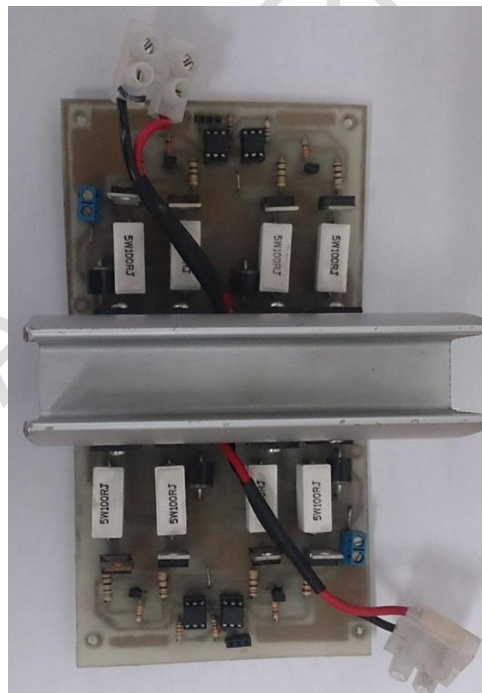
Figure 17. The H bridge implemented.
