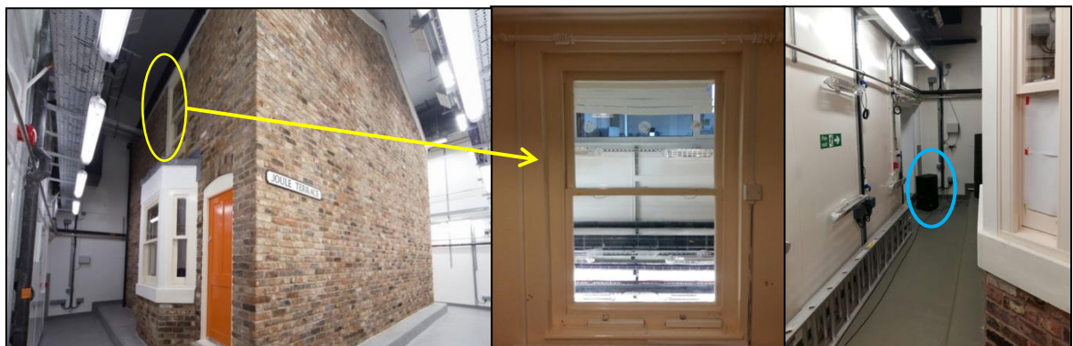
Figure 1: the energy house (left), the window tested (centre) and the loudspeaker in the house compound (in blue, right)
