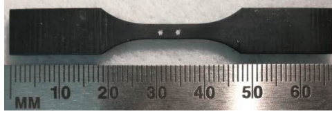
Figure 3.2 Typical Viton specimen cut from a larger sheet using an ASTM D638-V die.
