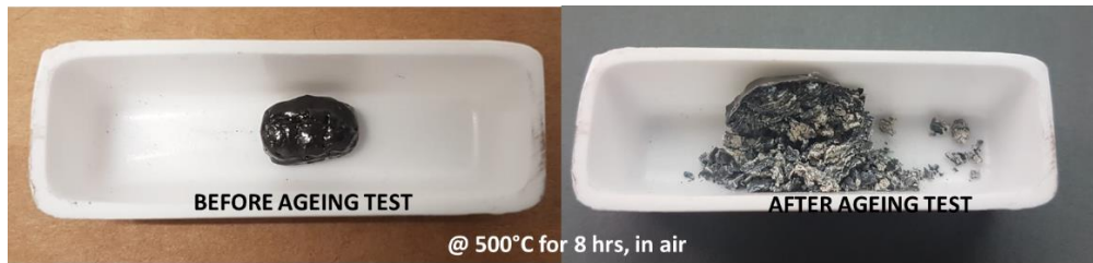
Figure 4.2-18: M5 glass coated \text{Mg}_2\text{Si}_{0.487}\text{Sn}_{0.5}\text{Sb}_{0.013} before and after the ageing test in oxidative atmosphere at 500^\circ\text{C} . After only 8 hrs the sample was exploded
