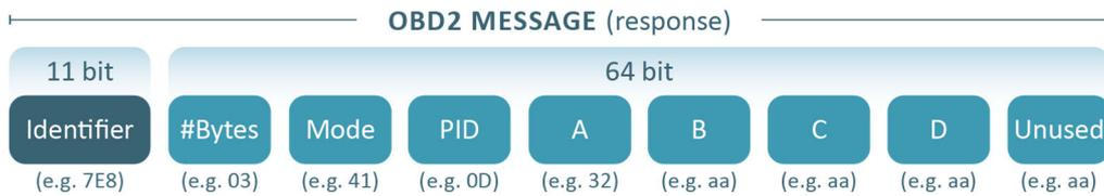
Figure 34. Typical structure of an OBD response message (source: [www.csselectronics.com](http://www.csselectronics.com))
