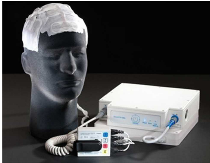
Figure 1.11: The NovoTTF-100A non-invasive alternative electric field application system 79 .
