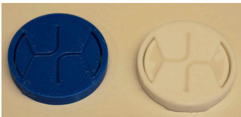
Figure B.11: Prototyping inserts by 3D printing. (Left) The ABS prototype made by FDM method; (Right) A prototype made by powder fusion method.
