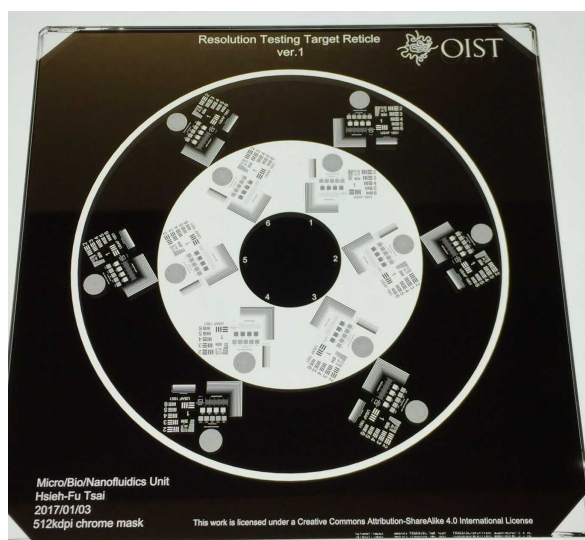
Figure D.6: A resolution testing reticle.
