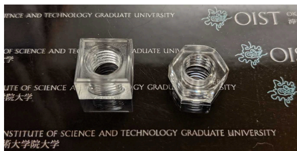
Figure 2.4: Disposable adapters for HPLC fittings 379 . (Left) A PMMA adapter with 1/4–20 thread; (Right) A polycarbonate adapter with M6 thread.
