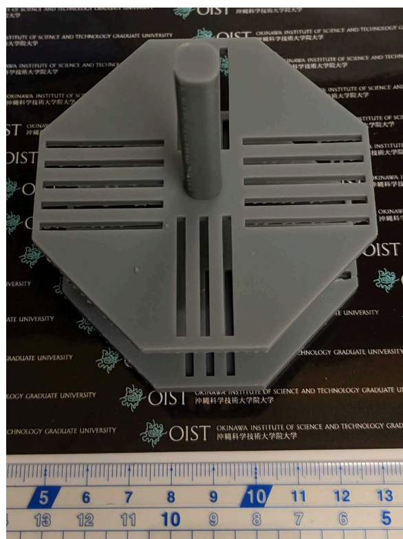
Figure D.3: The 3D printed washing stand for cover glasses.
