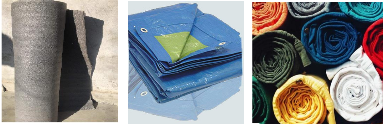
(a) Cellular polyethylene foam (12 mm) (b) Tarpaulin sheet (2 mm) (c) Fabric (10 mm)
