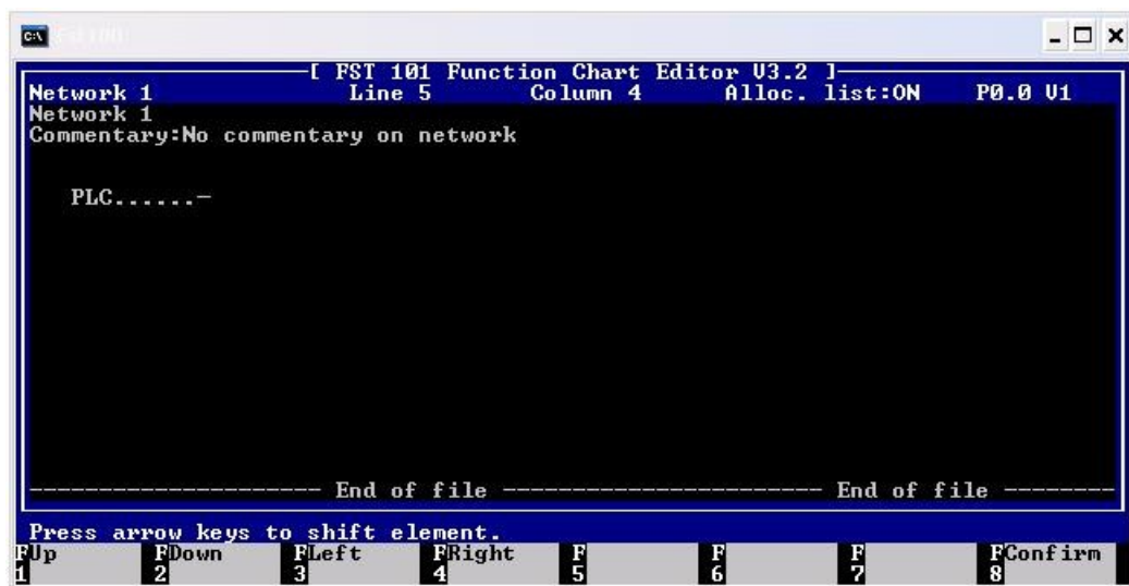
Gambar 3.32 Tampilan Command Shift Element .
