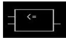
Gambar 3.30 Simbol Equal or Less Than .
