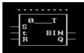
Gambar 3.18 Simbol Timer Switch-off Delay .
