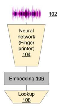
Fig. 1: Using a neural network to generate an embedding that enables matching a probe audio track to audio tracks in a database
