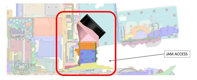
The solution explained in this disclosure allows access to the printzone area with one user interaction (pressing a button) and has optimized the cost of the movement of a mobile beam that needs position repeatability.
