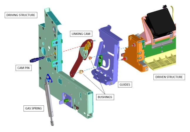
The driving structure is attached to the driven structure through linking cams. These linking cams are attached to the driving structure by the cam pins. Both structures can have different movement paths. In this specific case the driving structure has a translational circular movement defined by a parallelogram and the driven structure follows the guides path. The driving structure movement is triggered by a button or latch. In this case, a passive lifting system is used.
