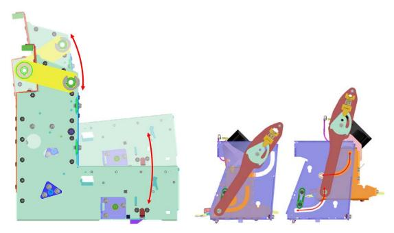
The guides path shape can be customized for the needs of the structure for service, clearance, etc... The paths help the driven structure avoid obstacles before rising up for the jam removal access. In this specific case, the driven structure has accumulated ink inside, and the paths avoid any possible ink spills by enforcing translation without rotation.
