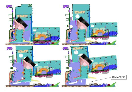
The guides paths are designed so that it cannot be automatically blocked by its own movement. To do this, the linking cam is always pushing or pulling in the guide general direction.
