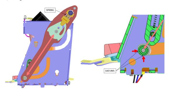
For assembly and service purposes, both movements can be unlinked to access both structures. In this case the lock/unlock system is made by a lever that unloads the spring against the cam pin, allowing its removal. This lever can be accessed from the outside of the printer with an allen key, so it makes it easy for the service technician to unlink the movements and access the structures.
