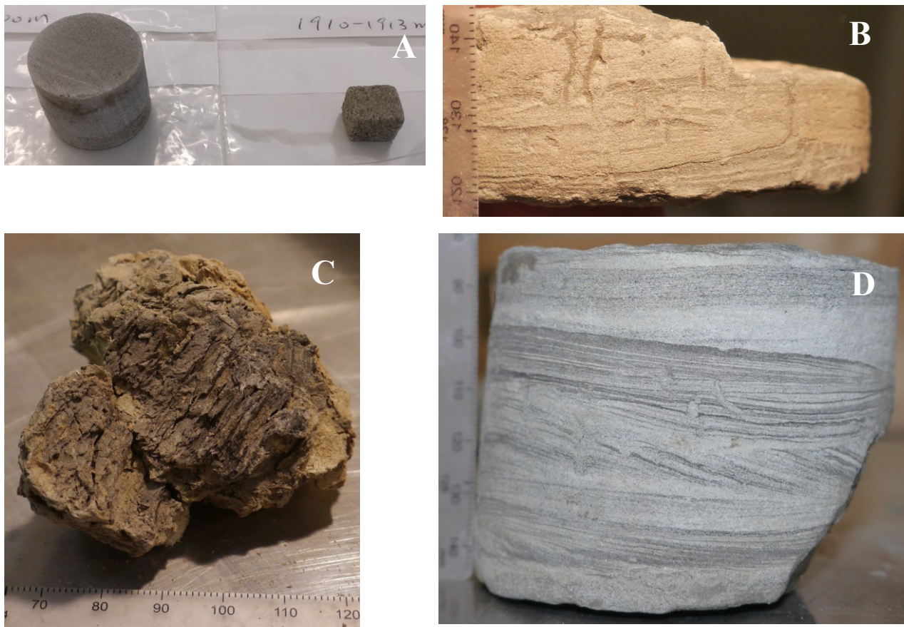
Figure 2: (A) Core samples from the nearby Kondoros-1 (Kond-1) well (Figure 1) from 1500-1900 m depth, prepared for XCT porosity scanning and flow through experiments. (B) Fine laminated sandstone core sample with rootlets interrupting ripple structures from Gyoma-1 well at 1990-1995 m depth. (C) Light grey to green Marl and grey silt laminations in a unconsolidated core fragment from Kond-1 well at some 1500 m depth. (D) Thin light grey laminated sandstone with small burrows intersecting dark grey lignite-rich laminations.
