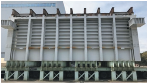
写真 11 鋼製土槽 Photo 11 Steel soil container.
