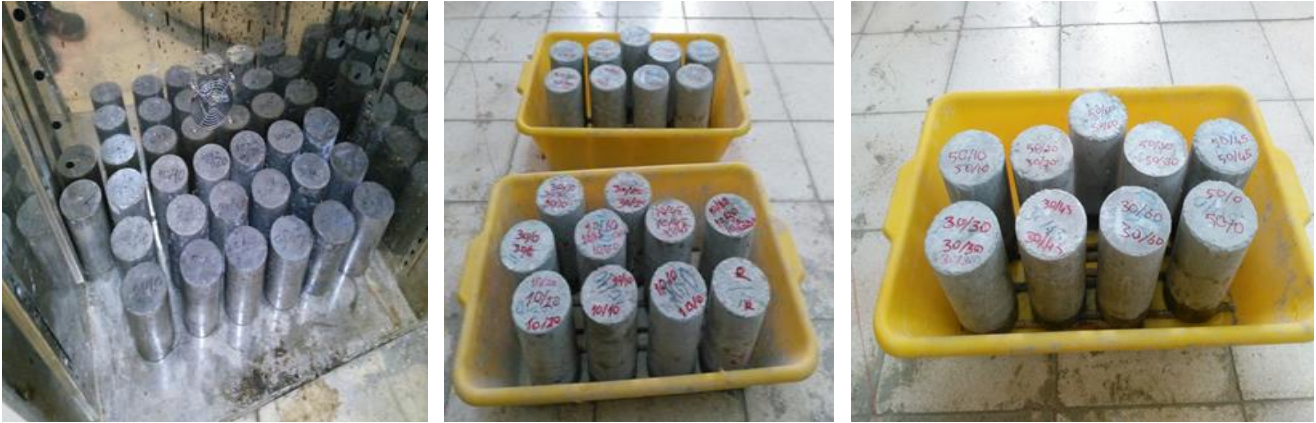
Fig. 6. Holding the concrete samples in the water filled container in the installed order.
