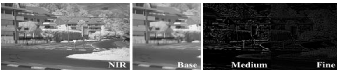
Fig. 2 Image decomposition by WLSF
