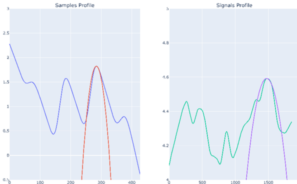
Fig 27. Image of wave profiles from both sample and signal dimensions. These profiles have been extended and fit with parabolas to mimic “perfect” wave propagation. Ideal waveforms resemble mass spectrometry readings, imaged above.
