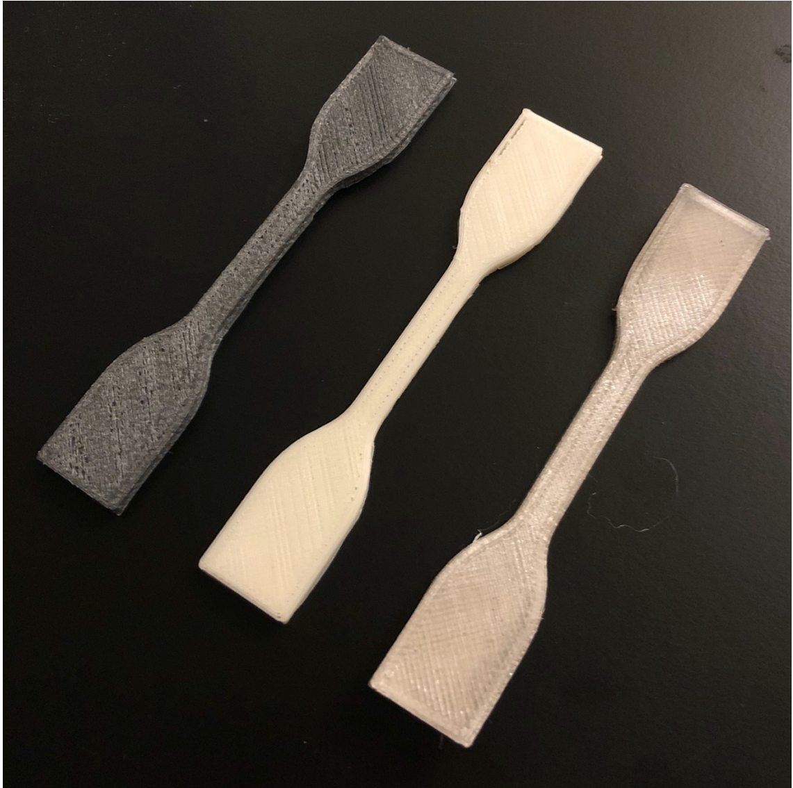
Fig. 14: Photograph of the 3D printed dog bones that are used to run tension tolerance tests and other mechanical tests to examine the properties of 3D printed thermoplastics. The dog bones (from left to right) are made out of acrylonitrile butadiene styrene (ABS) modified with 0.64% 1,6-bismaleimido-hexane functionalized graphene, base acrylonitrile butadiene styrene (ABS), and polycarbonate (PC). All filaments used to print these materials were produced using pellets that had been heated and extruded by a Filabot EX2 in order to make printable filaments.
