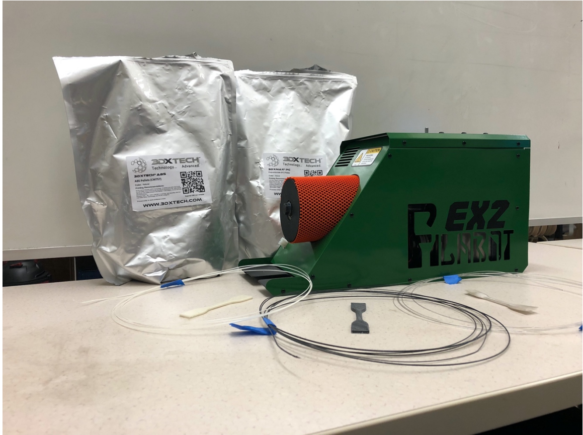
Fig. 13: Image taken at the NNF facility showing the Filabot EX2 used for filament production, the ABS and PC pellet bags used during filament production, and (from left to right) filaments of ABS, ABS modified with 0.64% 1,6-bismaleimido-hexane, and PC. The “dog bone” prints produced using each filament are also placed with their respective filament. These prints will be discussed below.
