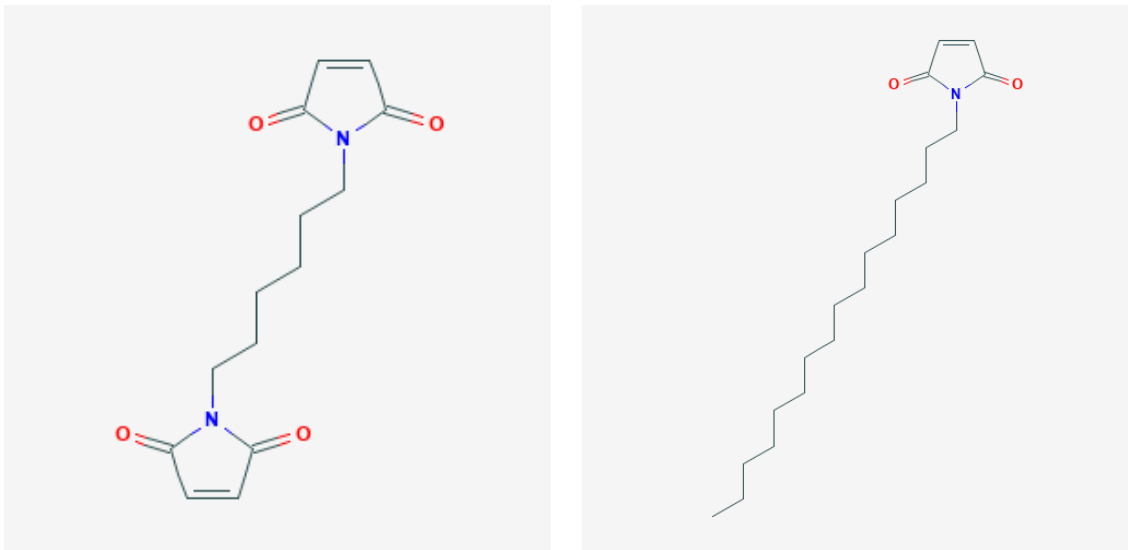
Fig. 6: (Left) 2D structure of 1,6-bismaleimidoheptane, which was used to modify the second sample of carbon fiber, and to modify the graphene that was then used to modify the fourth sample of carbon fiber. From PubChem 2020a.
