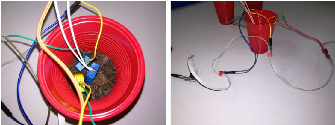
Fig. 2.21 Setup for impedance measurements with electrodes immersed in biofilter soil without bacteria
