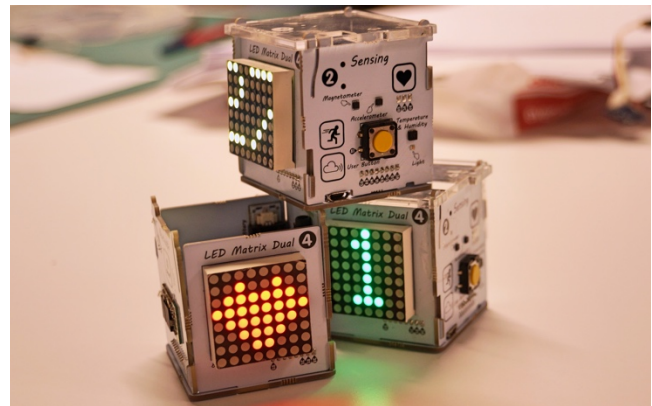
Figure 2: The Magic Cubes toolkit comprises hand-sized cubes with embedded sensors and collocated numeric or symbolic visualizations.
