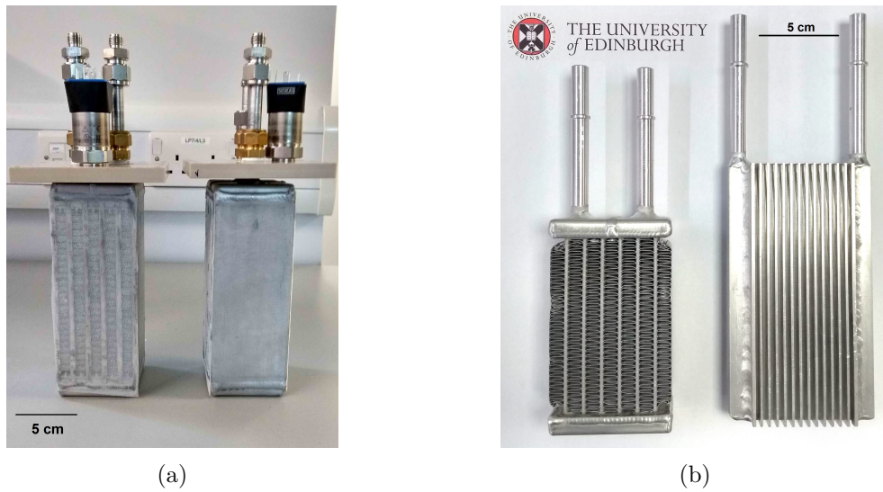
Figure 3: (a) Photograph of the front and side of the aluminium heat exchangers packed with silica gel, which is secured by the mesh. PEEK plates, pressure transducers, and fittings are mounted on top of the heat exchangers. (b) Photograph of the aluminium heat exchangers used for evaporator (left) and condenser (right).
