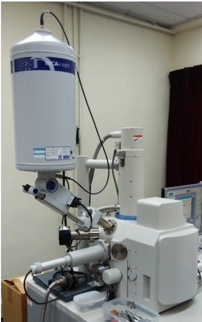
Fig. 3. Test setup for scanning electron microscopy analysis.
