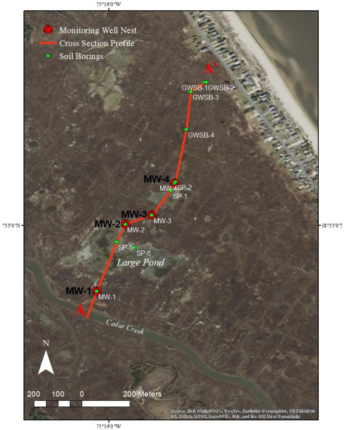
Figure 5: Detailed map of study area, showing locations of piezometer nests and sediment core locations used to construct the stratigraphic cross section.
