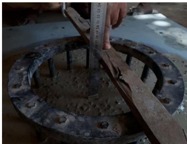
Figure 7. Pictorial views of slump flow and J-ring tests
