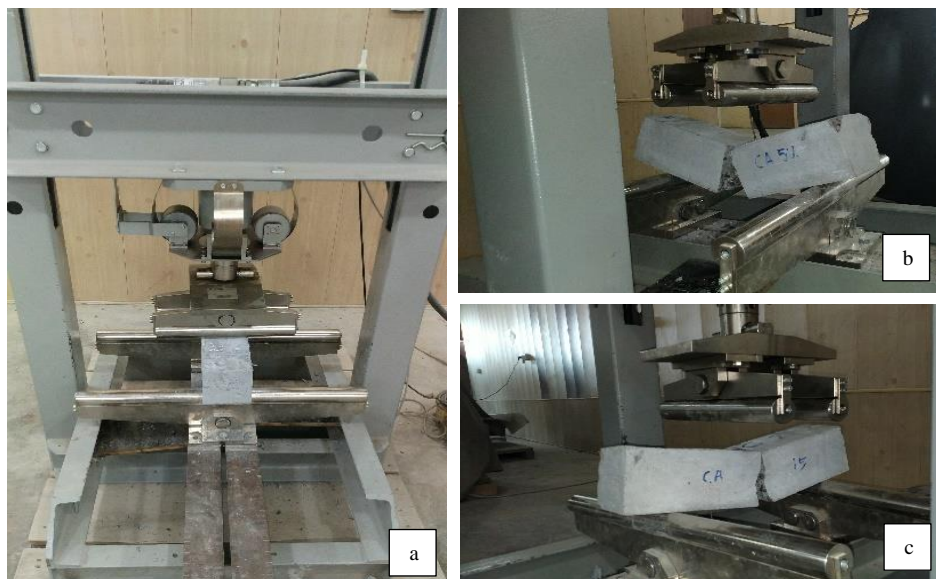
Figure 11. Modulus of Rupture test: (a) Flexural test machine, (b) Concrete prism with 5% chip rubber replacement, (c) Concrete Prism with 15% chip rubber replacement
