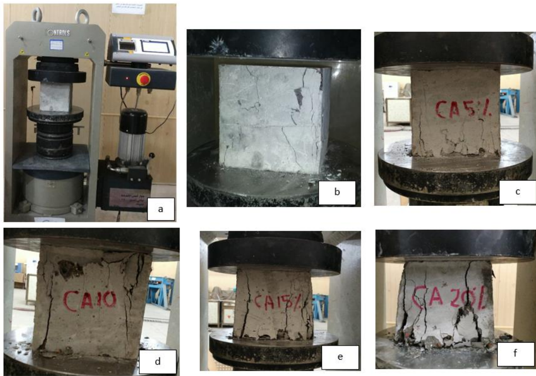
Figure 7. Tests of concrete cubes: (a) Compressive strength test machine, (b) Cube with normal concrete, (c) Cube with 5% chip rubber replacement, (d) Cube with 10% chip rubber replacement, (e) Cube with 15% chip rubber replacement, (f) Cube with 20% chip rubber replacement.
