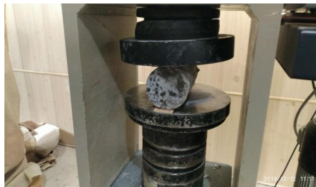
Figure 9. Splitting tensile test
