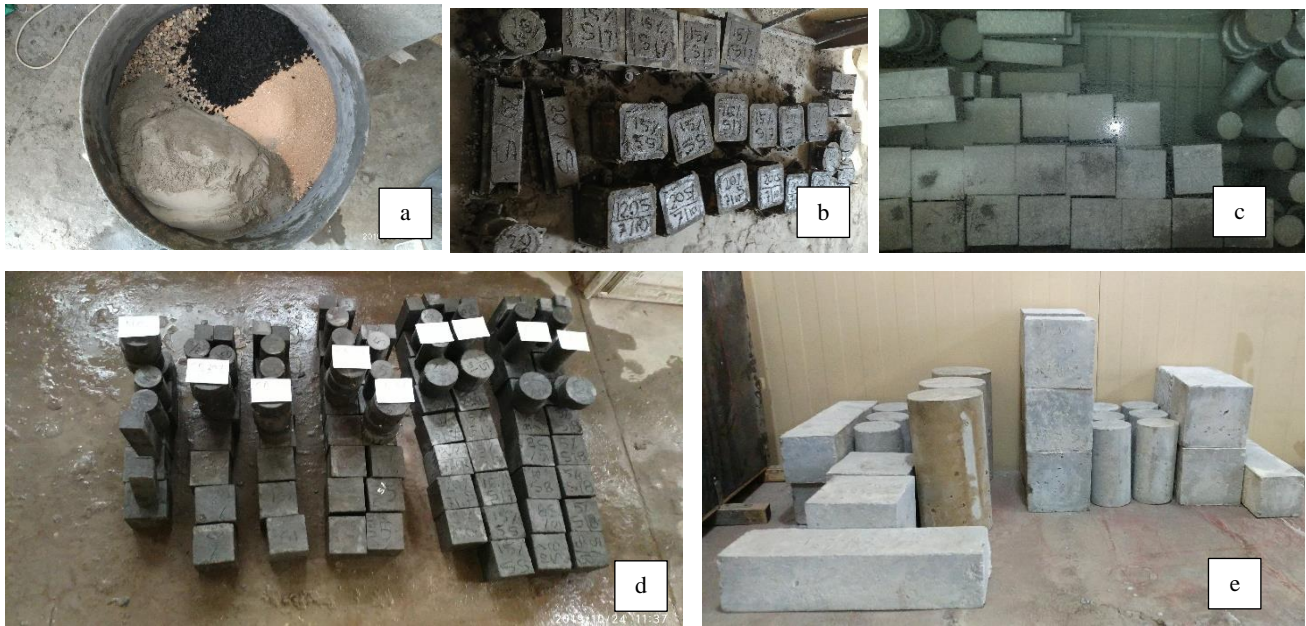
Figure 5. Preparing specimens: (a) Mixing materials, (b) Specimens casting, (c) Specimens curing, (d and e) Preparing specimens for test
