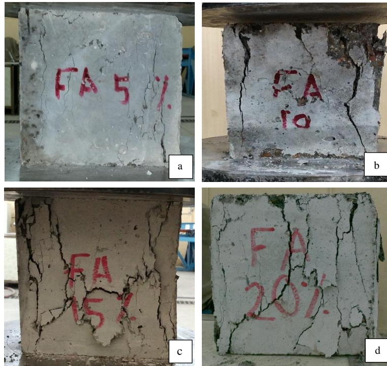
Figure 8. Tests of concrete cubes: (a) Cube with 5% crumb rubber replacement, (b) Cube with 10% crumb rubber replacement, (c) Cube with 15% crumb rubber replacement, (d) Cube with 20% crumb rubber replacement
