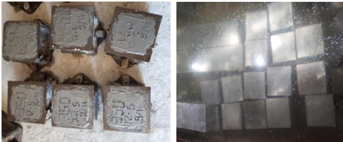
Figure 2. Filling moulds with concrete mixture and Specimens Curing
