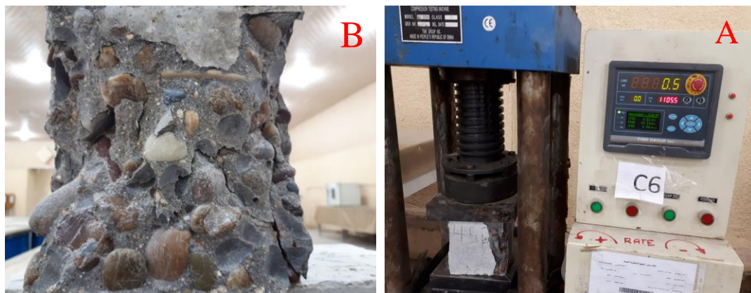
Figure 5. Failure mode of a sample of normal; Strength, concrete with MSCA (37.5 mm)
