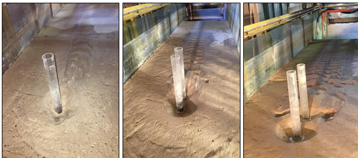
Figure 4. Sediment deposition at the downstream of the scour hole for the case of single pier and two inline piers with different spacing
