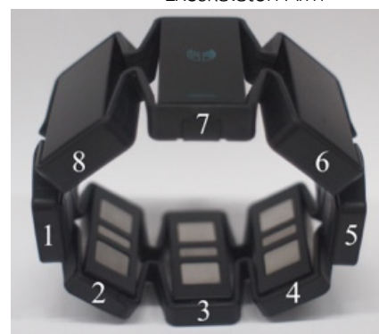
Figure 2 Number of Electrodes on the MYO Armband
