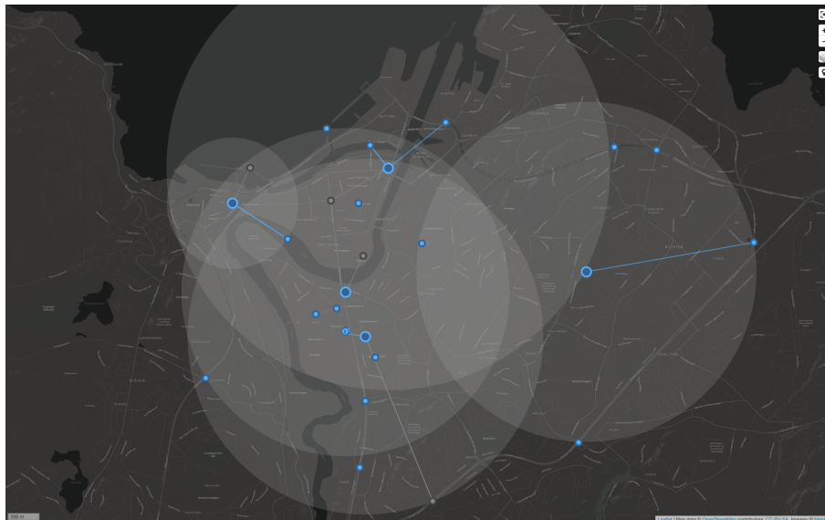
Figure 8: Visualization of an initial network of two installed gateways and two nodes with additional simulated gateways and sensor nodes, dataflow and coverage
