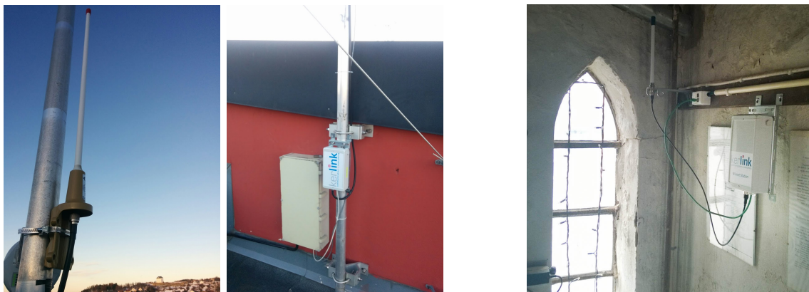
Figure 5: Deployment of LoRaWAN antenna gateway outdoors on the roof of the Student Society building in Trondheim (left) and elevated indoors in a clock tower in Vejle (right).
