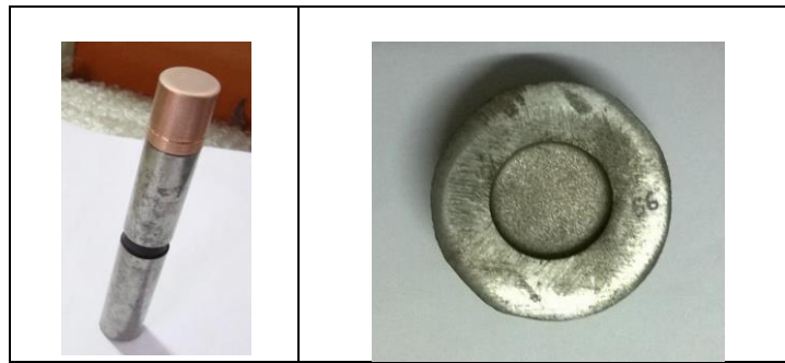
Fig. 3 Round copper tool and machined component (5 mm depth and 20 mm dia.)
