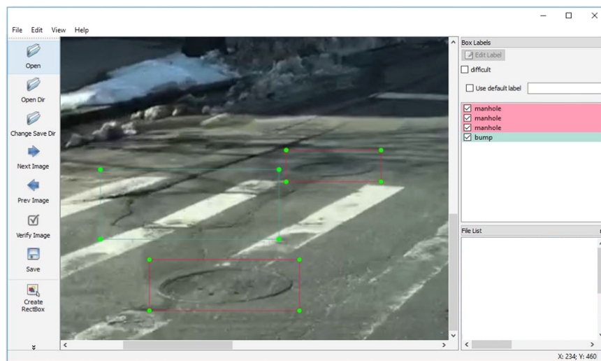
Figure 7: Image annotation using 'labellmg'.
