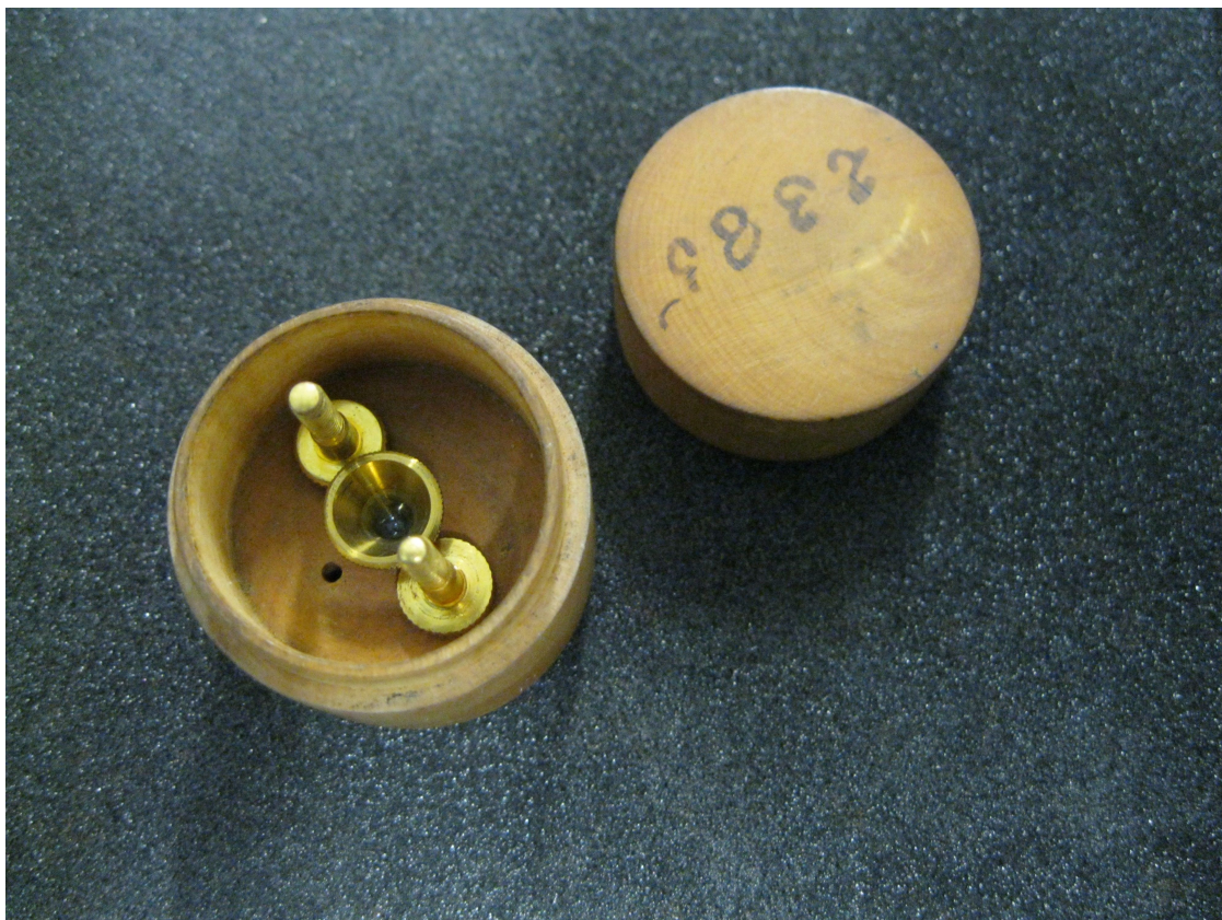
Figure 6.10: Sapphire cup and iridium tipped pivot (point down), 1837-40, AC00972, Greenwich National Maritime Museum, Greenwich, London.
