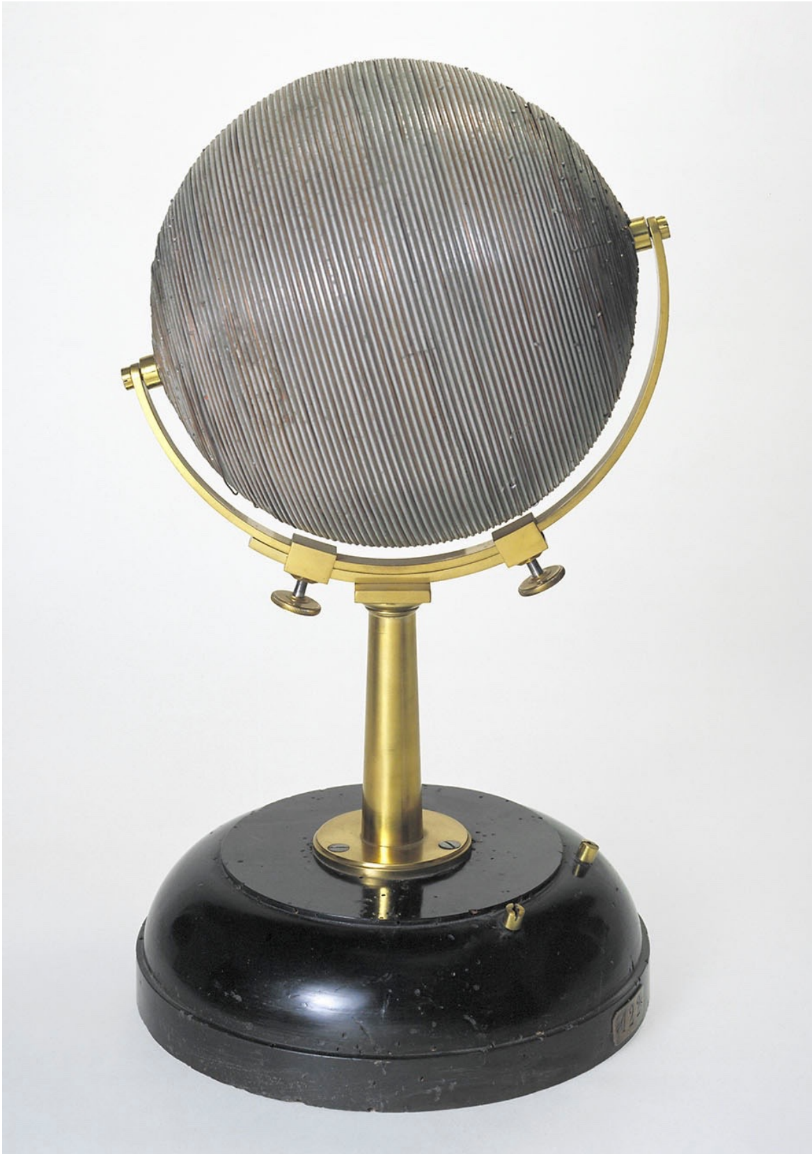
Figure 3.11: a c.1830 edition of Peter Barlow's 1824 globe, commissioned by Italian physicist Leopoldo Nobili. As with Barlow's the globe is made of wood tightly wound in copper, 413, Museo Galileo
