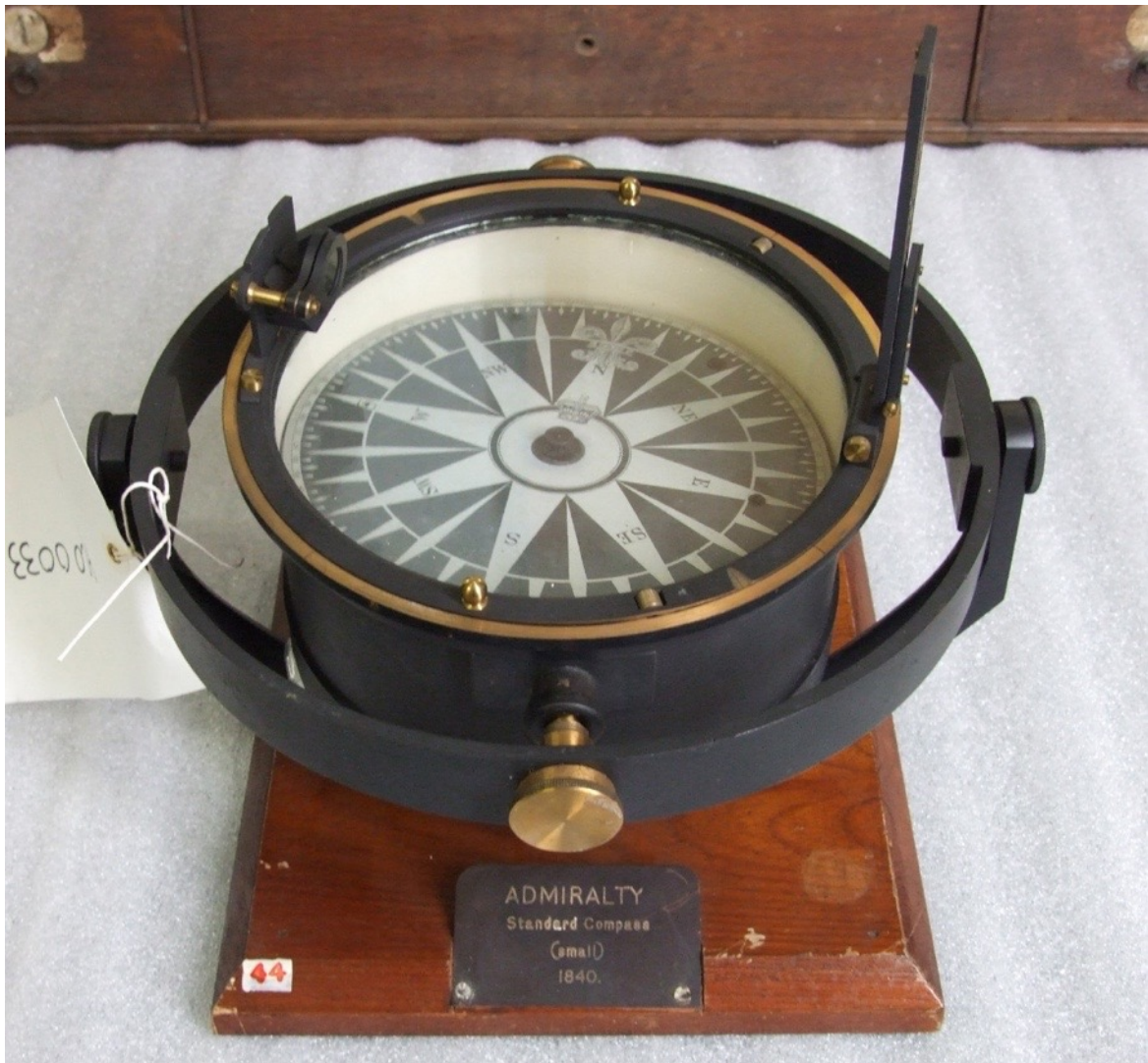
Figure 6.8: Admiralty Standard Compass, adapted for small ships 1840, ACO0033 Greenwich National Maritime Museum, Greenwich, London.
