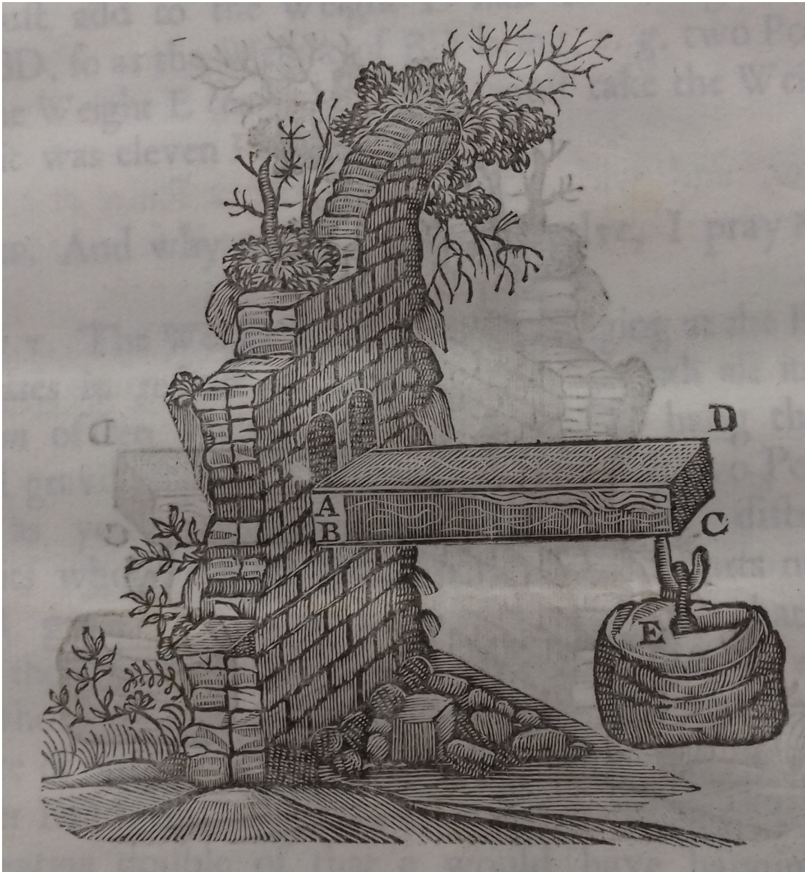
Figure 3.4: Galileo's cantilever model, Galilei, Galileo, 1730, Mathematical Discourses concerning Two New Sciences relating to Mechanics and Local Motion... done into English from the Italian by Thomas Weston , London: J. Hooke, pp.169-70.
