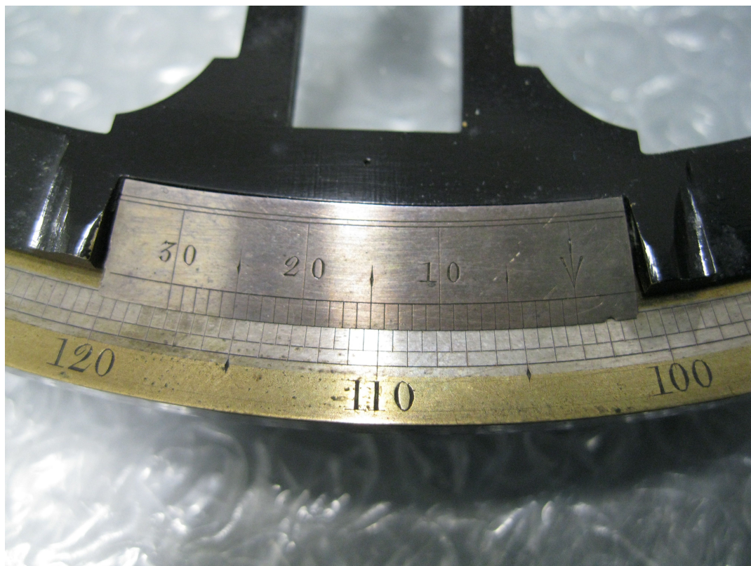
Figure 6.13: silver scale set into the verge of the azimuth ring, ACO1363, Greenwich National Maritime Museum, Greenwich, London.
