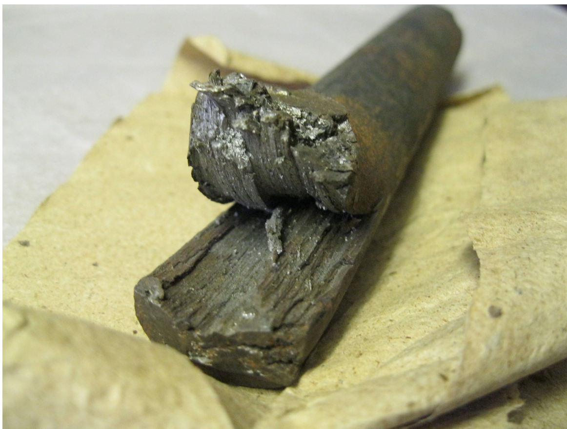
Figure 3.3: 'No.4: A portion of a bar of Fibrous Iron which was placed on the top of a Tilt hammer working at the rate of 355 strikes per minute & which after being exposed to this species of concussion for 24 hours at last broke off quite short like a piece of glass' c.1840, WHITMSCO178, Whitby Museum.
