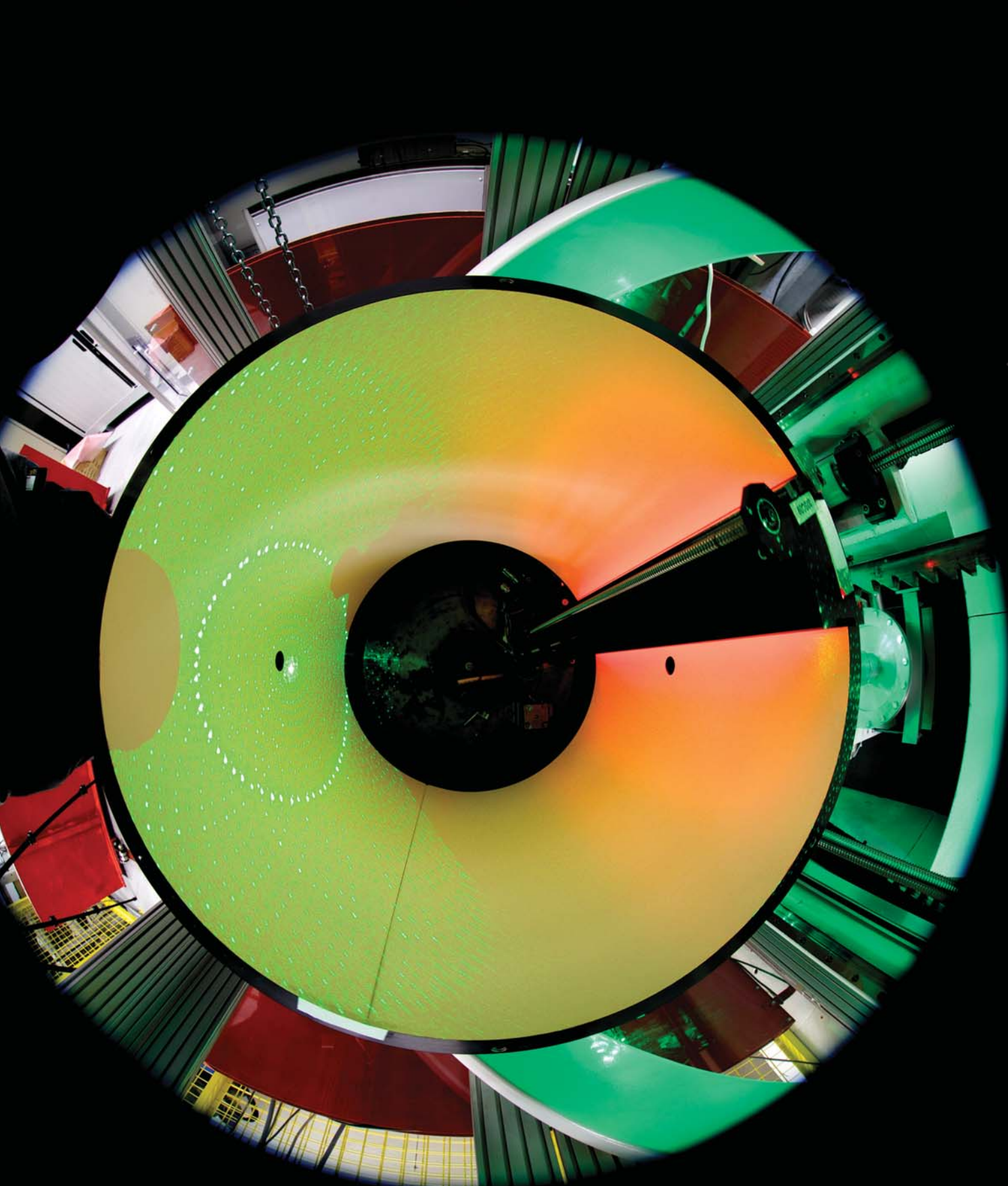
A cylindrical detector in the LADI instrument at the Institut Laue-Langevin in Grenoble, France, records neutron diffraction patterns. The data enable the generation of three-dimensional molecular structures that include hydrogen atoms. (Bob Cubitt/ILL.)
