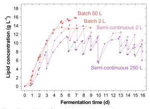
**Fig. 6** The scalability of *Metschnikowia pulcherrima*. Comparison of the lipid concentration in *M. pulcherrima* cultures when grown batch-wise or semi-continuously on glucose syrup on the 2-, 50- or 250-L scale in stirred tank reactors. A constant gas volumetric flow rate was used as scale-up criterion and linear scale-up parameters kept constant for each batch and semi-continuous operation as base for scale comparison [29]
