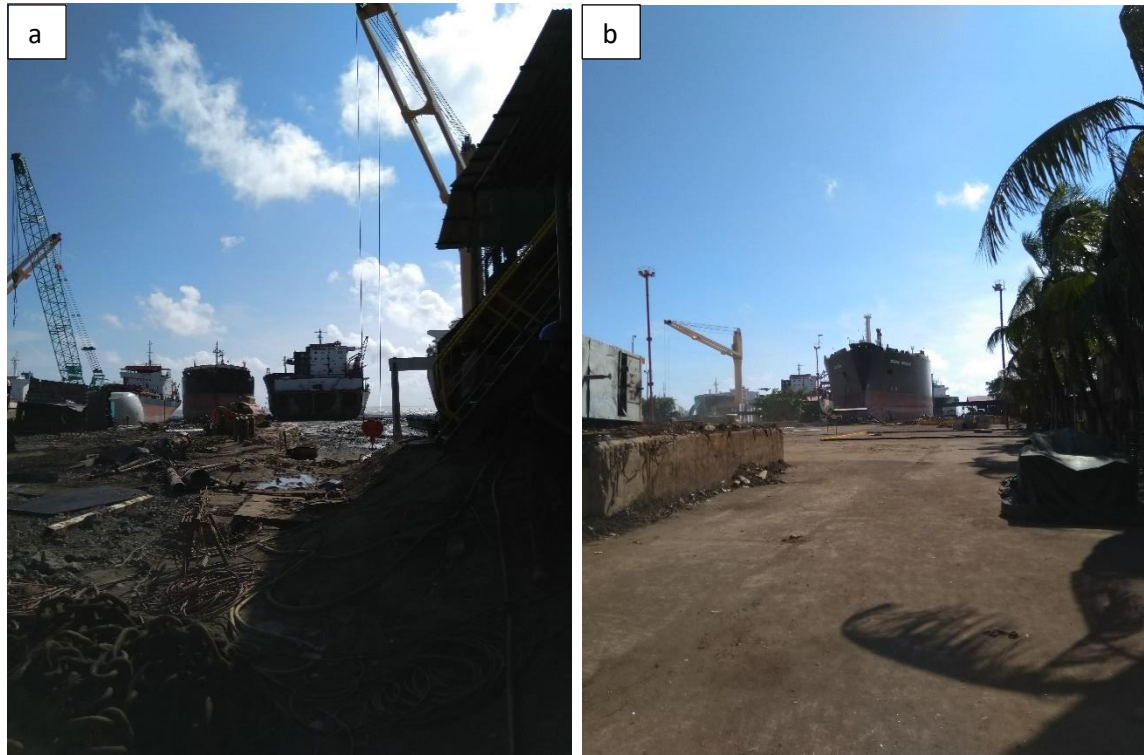
Figure 5: One of the shipbreaking yards in Chittagong, Bangladesh showing (a) the primary cutting zone and (b) the secondary cutting zone (i.e. materials processing zone).
