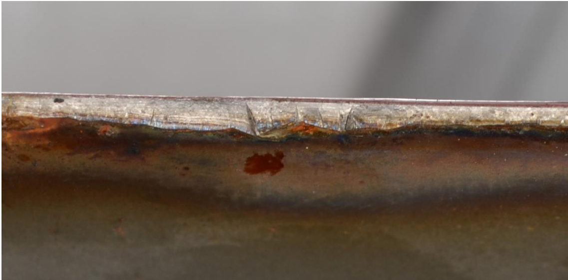
Figure 4 The fracture surface showing evidence of blue and straw temper colours, proving that the crack originated as a hot crack during solidification.
