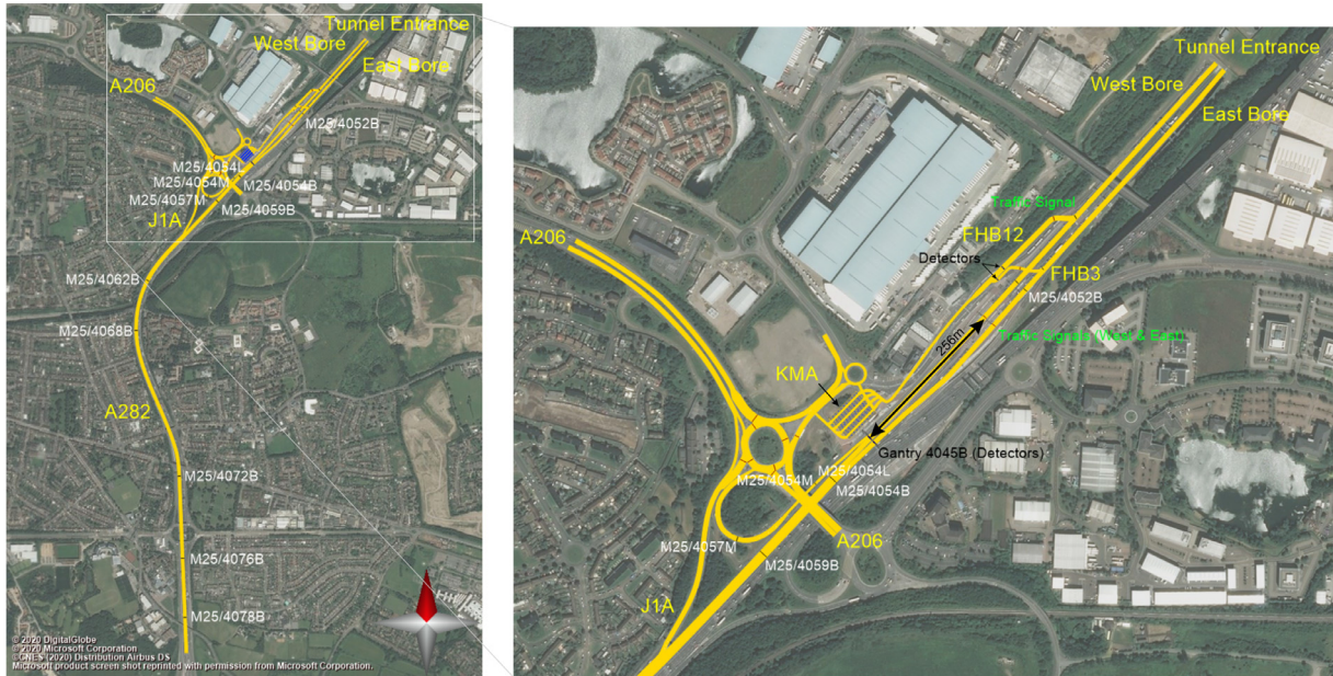
Fig. 1. PTV Vissim model highlighting key roads, detectors, and traffic signal locations at the Dartford Crossing.
